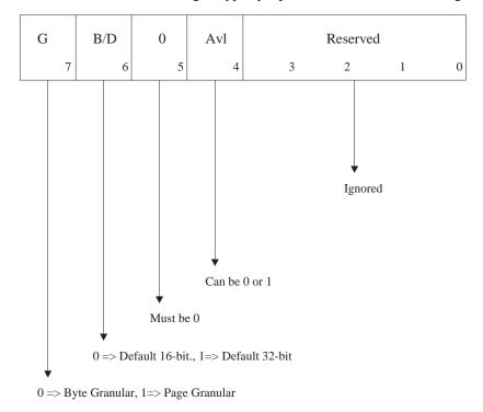
The extended access rights/type byte passed in CH has the following format.
