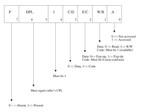
The access rights/type byte passed in CL has the format shown in the figure below.
